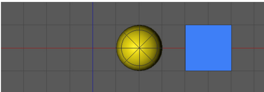
Figure 10 – after mirroring with local coordinates, the sphere is at local X -300, global +200
